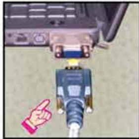
Connect VGA cable to laptop monitor output. NOTE: SOME LAPTOP MODELS MAY REQUIRE ADAPTORS.
