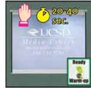
Allow projector to warm up LOGO DISAPPEARS, READY LIGHT IS ON, WARM-UP LIGHT GOES OUT.
