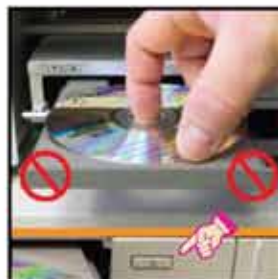
Load disc, press OPEN/CLOSE button to close tray. DO NOT PUSH TRAY TO CLOSE!
